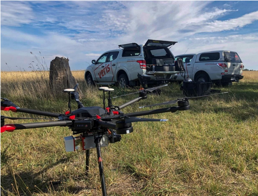
Figure 3: Riegl MiniVUX LiDAR UAV in preparation for takeoff.
