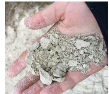
Figure 6. The bleached horizon of soils associated with the Werribee Formation is fine textured and fragile. Soil structure crumbles easily in the hand.
