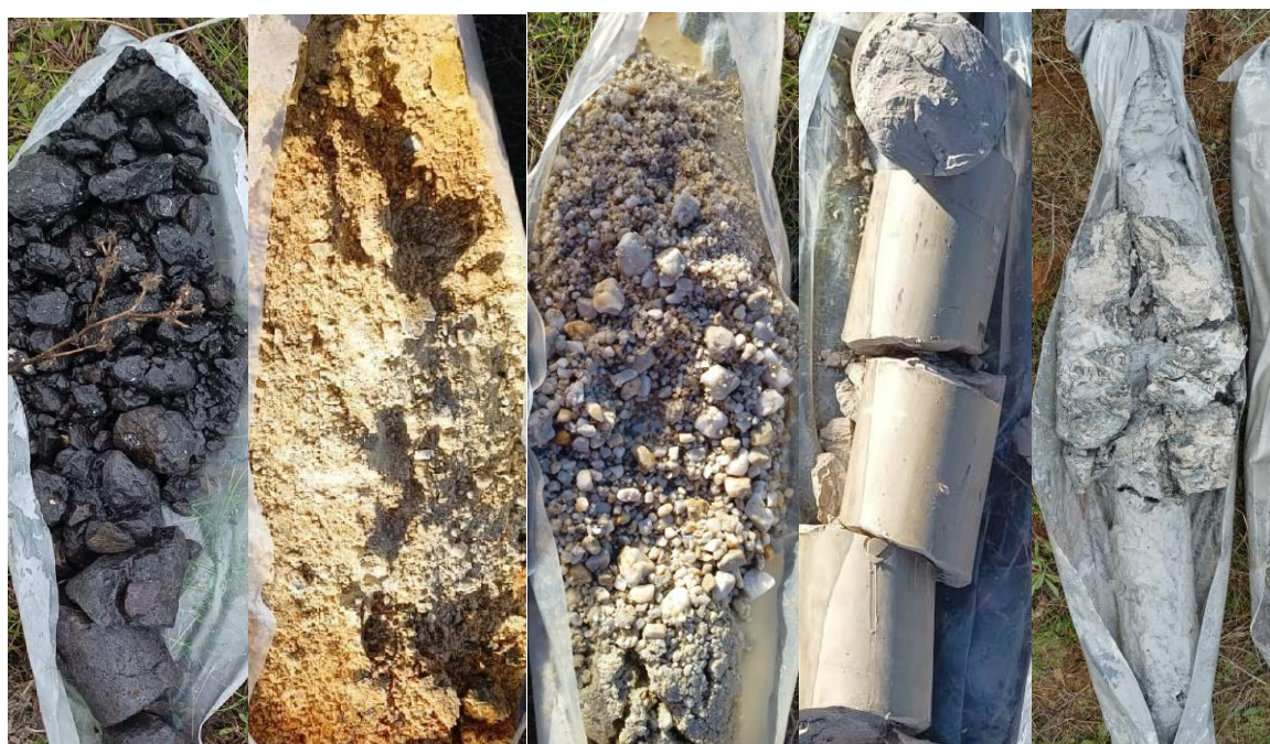
Figure 14. Left to right: Basalt, Werribee Formation sand, Werribee Formation gravel, Werribee Formation clay, Werribee Formation coal and Basement (siltstone).
