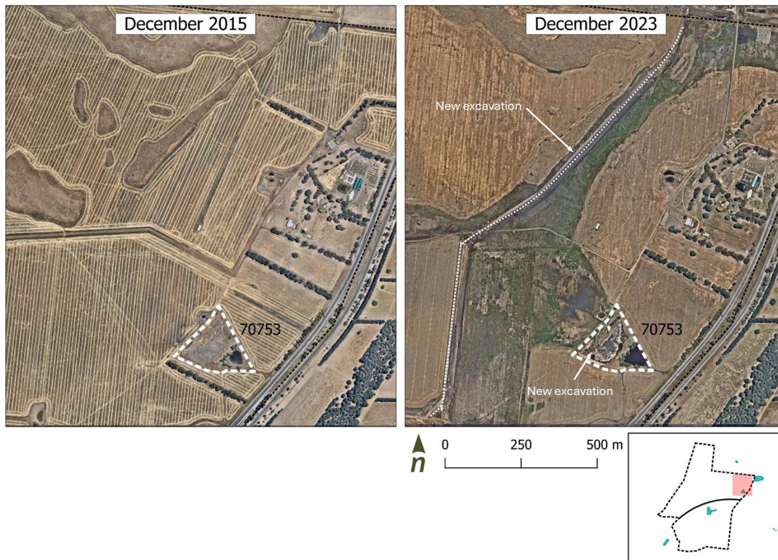
Figure 8. Aerial images of wetland 70753 from 2015 (left) and 2023 (right) with recent drainage line and wetland excavation annotated.
